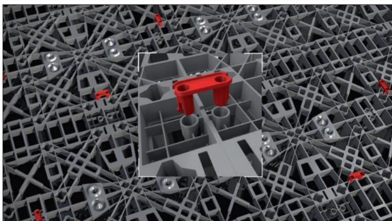
15.7 Subsequent layers are placed directly on top of the previous layer. The modules are aligned in the same direction, creating the inspection tunnel (see Figure 6). Installation lugs on the top and base of each module ensure that modules are installed in the correct orientation.
